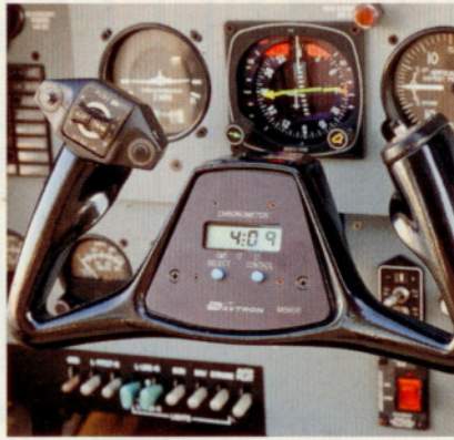
The panel is large enough to accommodate any avionics gear an owner might need (below). Big-airplane features include a beefy power control quadrant and an overhead panel. Note the airspeed indicator, which requires you to add a 0 for indicated airspeed. The tachometer reads engine rpm rather than prop rpm.
