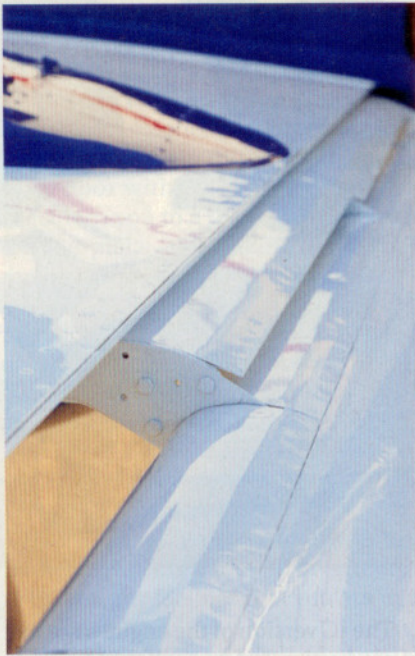
The double-slotted Fowler flaps allow the Beagle to fly at incredibly low speeds. Because of this, the Beagle can land on runways that it can't get out of. Notice the use of flush riveting for a smooth surface. That long, smooth wing is optimized for high speed and makes descent planning a challenge for Beagle pilots.
